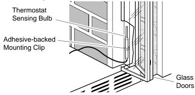
Figure 31 - Installing Thermostat Sensing Bulb behind Glass Doors
